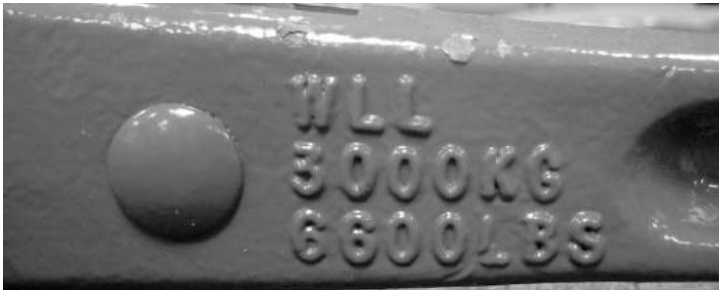
Indicator of Working Load Limit
